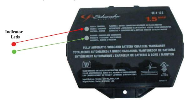
2. Connect the battery charger unit to a ll0VAC outlet. The red charge indicator LED will turn on solid to indicate that the charging unit is fast charging the battery.
