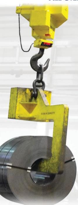
Model shown with optional head room loss adapter and AC operation.
